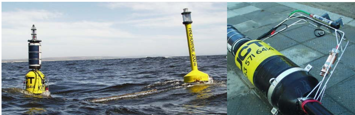
Fig. 5. The principal scientific (BOB) and marker buoys (BOMB) in position on the tight line mooring (left), and the upwelling radiance sensor arm on BOB (right). The scientific buoy has a payload of two Trios hyperspectral radiometers, a fluorometer, a thermistor chain, and an ADCP.
